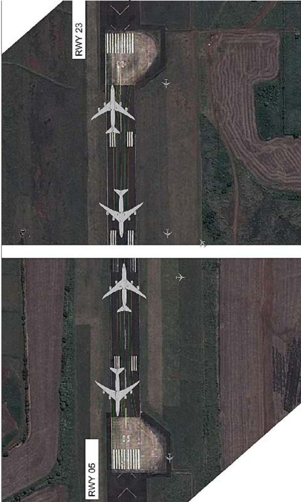
Chart VII: 747-8F U-Turn Analysis – RWY 05 and RWY 23 Turn Pads
