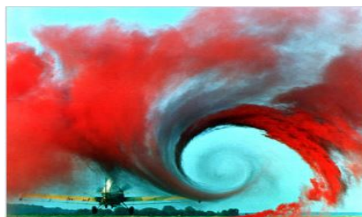
This picture from a NASA study on wingtip vortices qualitatively illustrates the wake turbulence.
