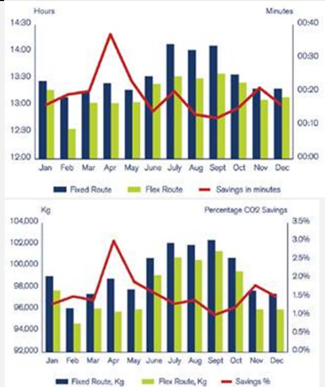
Comparison of Flight Time and Fuel Burn using Fixed and Flex Routes using Sao Paulo-Dubai flights throughout the year 2010 (Source: IATA iFLEX Preliminary Benefit Analysis)
