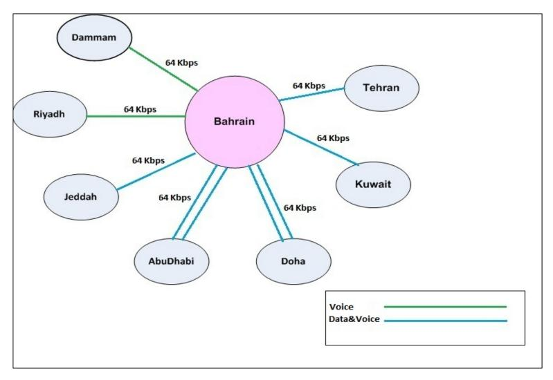
Figure 1: Bahrain Circuit Diagram
