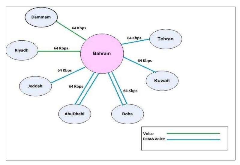
Figure 1: Bahrain Circuit Diagram
