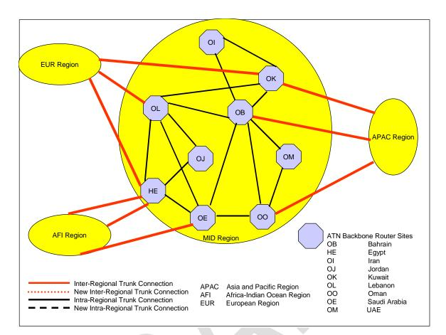
Figure 5-1 MID ATN Backbone Routing Architecture
