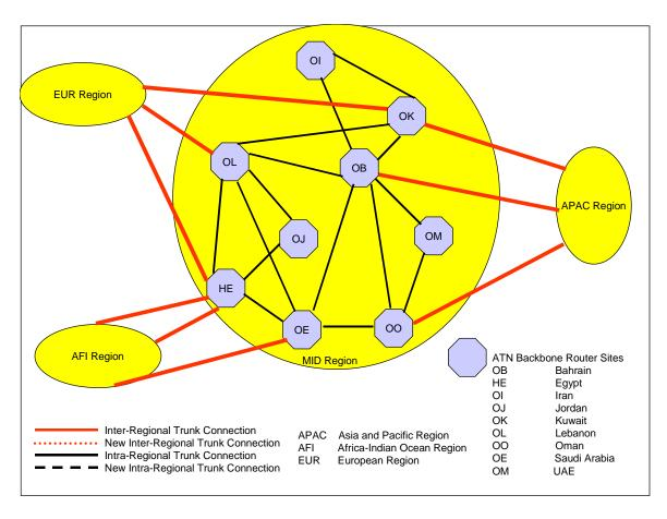
Figure 5-1 MID ATN Backbone Routing Architecture
