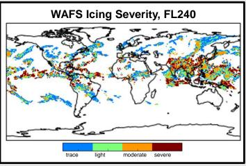
It can be seen that the new Icing Severity field contains much more distinct icing areas. More moderate/severe icing is forecast, particularly in the tropics; this is due to an improvement in the way convective icing is calculated.
