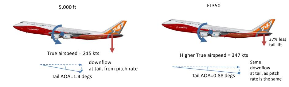
So, pitch damping is 37% less at the higher altitude, which makes it harder to control
