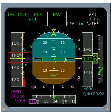
Current mode Mode transition AOA and its limit Speed trend and target Pitch limit indicators (some) Sideslip Descent rate Attitudes Flightpath
