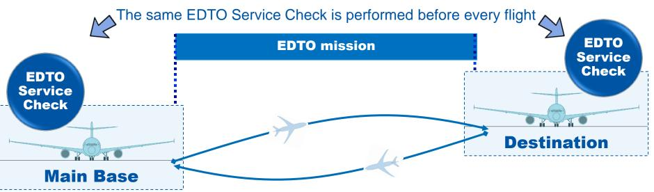
This approach of **single** EDTO <u>pre-departure</u> service checks may not be compatible with the flight program typically when the mission is a sequence of EDTO / non-EDTO legs.
