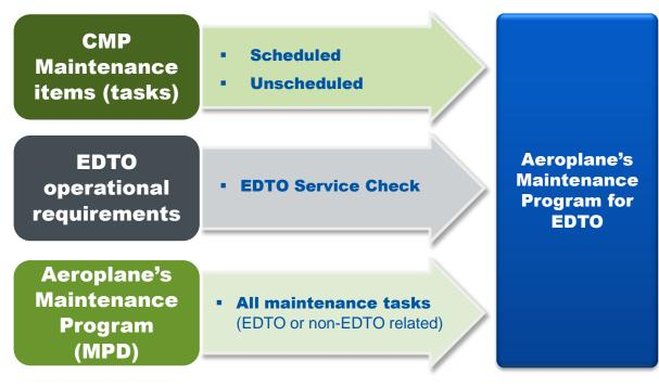
The aeroplane should be maintained in accordance with the **aeroplane's maintenance program for EDTO** as long as it is operated on EDTO flights.
