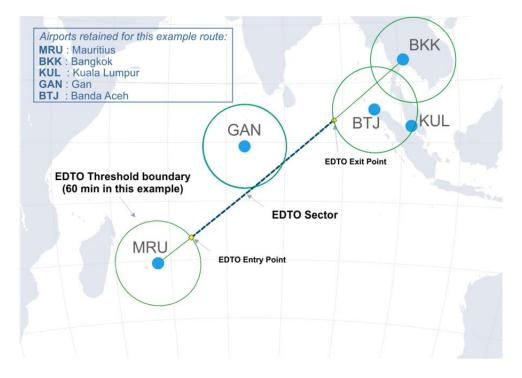
Figure 3.5-2b. Example of multiple EDTO sectors treated as a single sector
