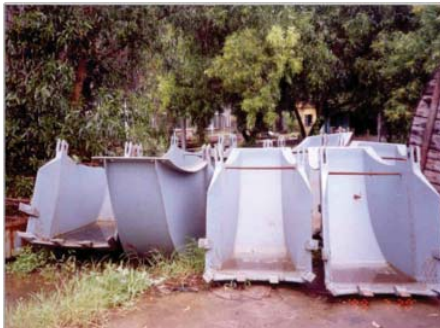
Figure 34. Mineral ore loader buckets with water accumulation © Ashwani Kumar
