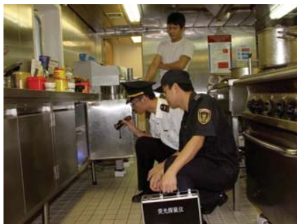
Figure 22. Shipboard inspection for rodent urine with UV light © Tianxiao Chen, Shenzhen Entry-Exit inspection and quarantine bureau, China.
