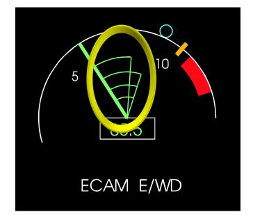
Low energy warning in approach Actual / commanded engine thrust
