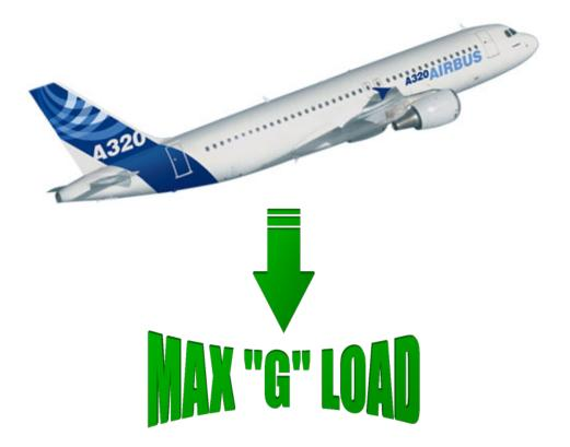
Should a sudden evasive maneuver be necessary, the G-load protection limits the load factor to +2.5 g
