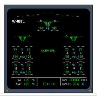
The ECAM system will automatically display the WHEEL SD page after the engines have been started
