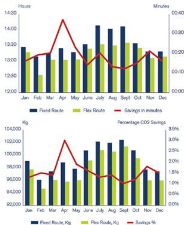
Comparison of Flight Time and Fuel Burn using Fixed and Flex Routes using Sao Paulo-Dubai flights throughout the year 2010 (Source: IATA iFLEX Preliminary Benefit Analysis)
