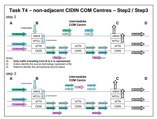
Figure 10: Task T4 - non-adjacent CIDIN COM Centres - Step2 and Step3
