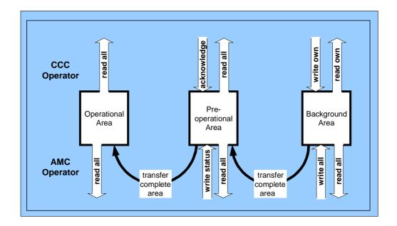
Figure 3: Schematic representation of the three Data Areas
