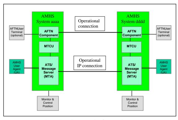
Figure 1: AMHS Pre-operational Test Environment
