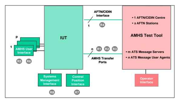
Figure 5: Generic test configuration with points of reference
