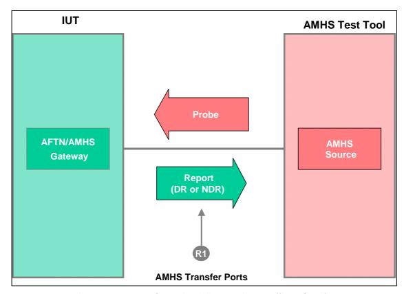
Figure 11: Test configuration "Gateway" – Handling of Probes
