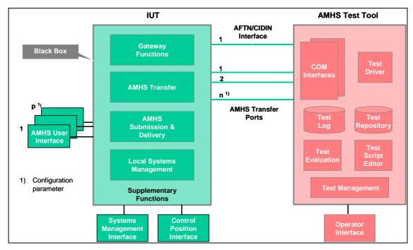
Figure 3: Model of the test environment
