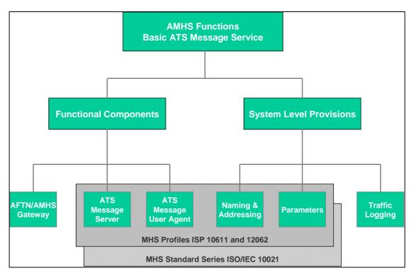
Figure 1: AMHS functionality specified by the AMHS technical specifications
