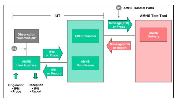
Figure 6: Test configuration "Submission"
