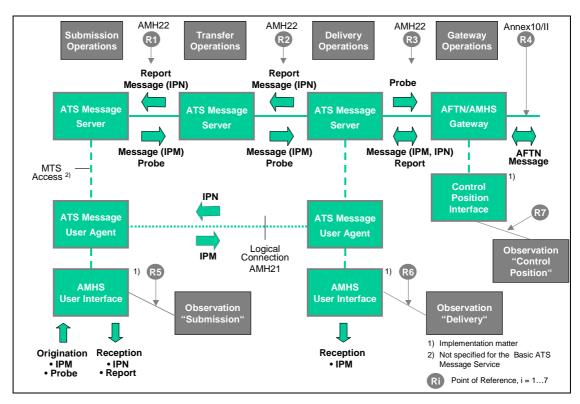
Figure 4: Generic AMHS communication scenario and used Points of Reference for conformance testing
