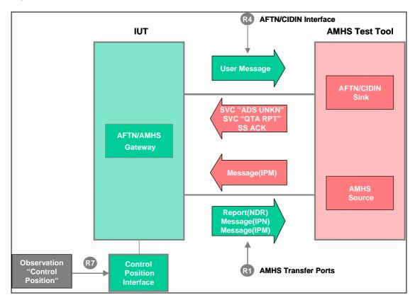
Figure 9: Test configuration "Gateway" – User message from AMHS to AFTN
