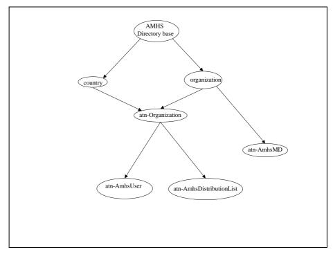
Figure 2: DIT structure for AMHS address conversion
