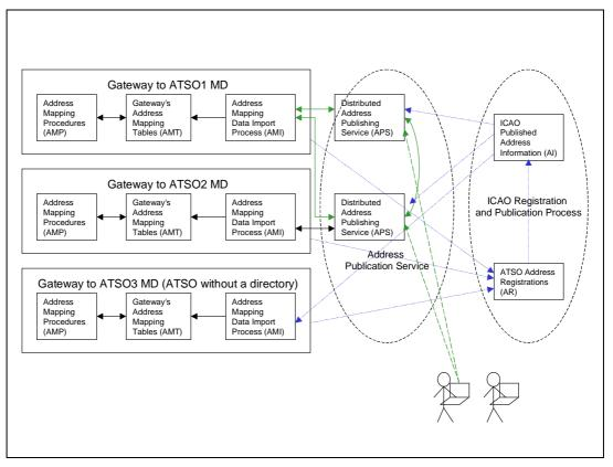
Figure 1: General model for gateway address conversion
