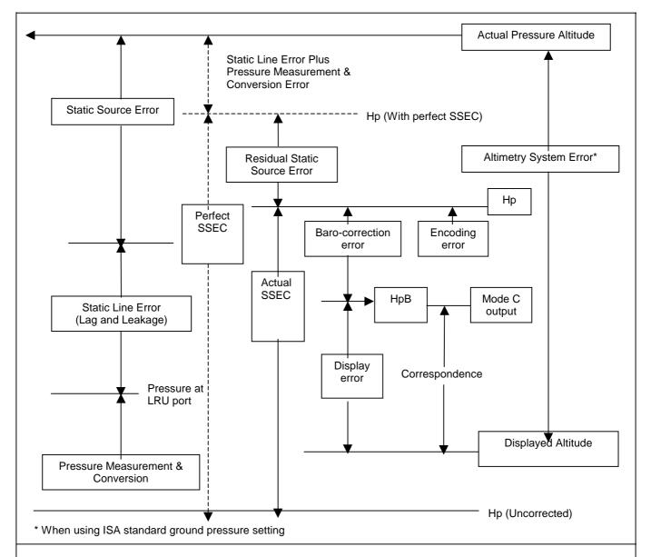
(f) 'Residual Static Source Error' is applicable only in systems applying an avionic SSEC. It is the difference between the SSE and the correction actually applied. The corrected value of Hp will therefore differ from actual pressure altitude by the sum of static line error, pressure measurement and conversion error, and residual SSE.
