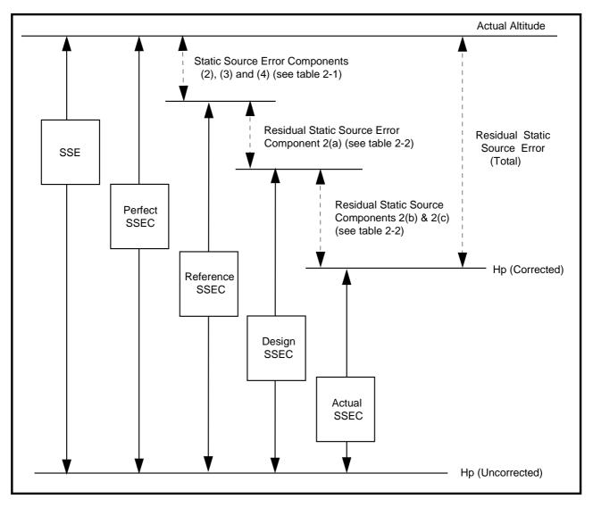
3.2.3 *Static Line Error* Static line errors arise from leaks and pneumatic lags. In level cruise these can be made negligible for a system that is correctly designed and correctly installed.
