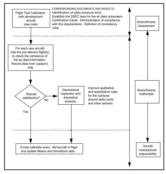
Note : The flight test installation chosen to get the calibration data will need to have an accuracy compatible with the level of performance to be demonstrated and an analysis of this accuracy will need to be provided. Any possible degradation of this accuracy will need to be monitored and corrected during the flight test period.
