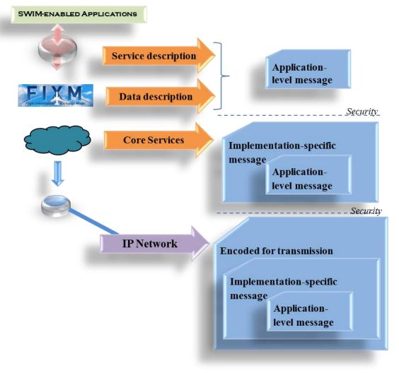
Figure 4. Layers encapsulate messages from prior layers
