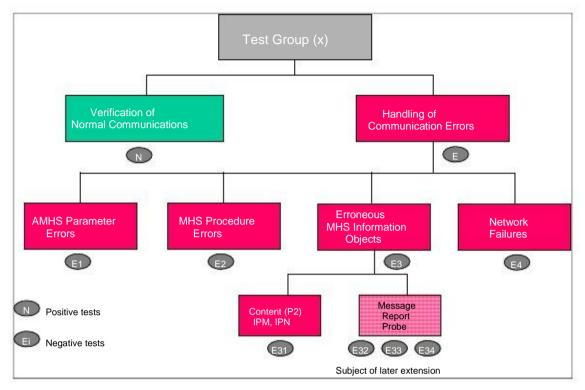
Figure 13: Classes of "Negative Tests"
