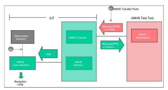
Figure 8: Test configuration "Delivery"
