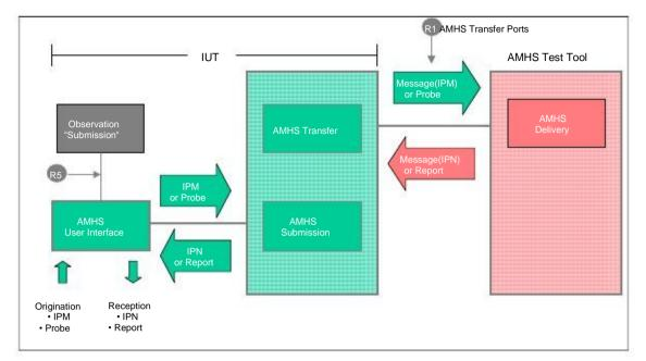
Figure 6: Test configuration "Submission"
