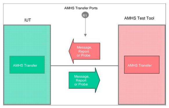
Figure 7: Test configuration "Transfer"
