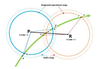
Figure 6. – SSR Mode S interrogator clustering (interrogators with same II code)
