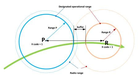
Figure 10. - Minimum separation distance between interrogators having the same II code
