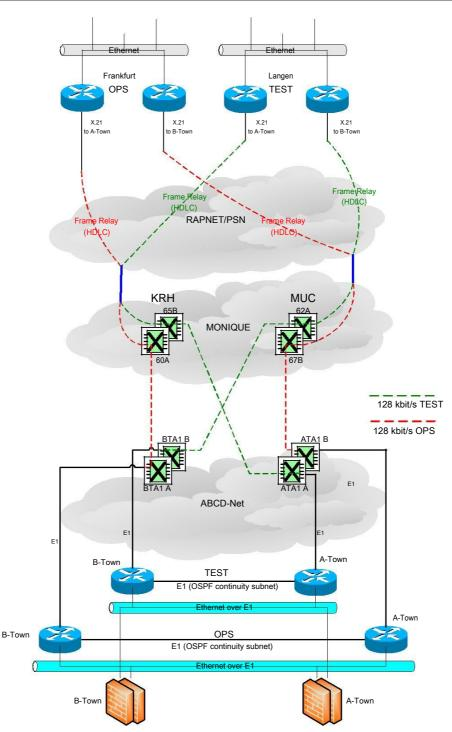
Figure 2: Example for a redundant international IP connection (Operational and Test)
