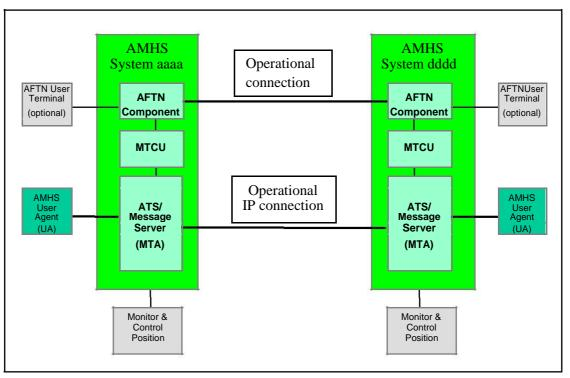
Figure 1: AMHS Pre-operational Test Environment
