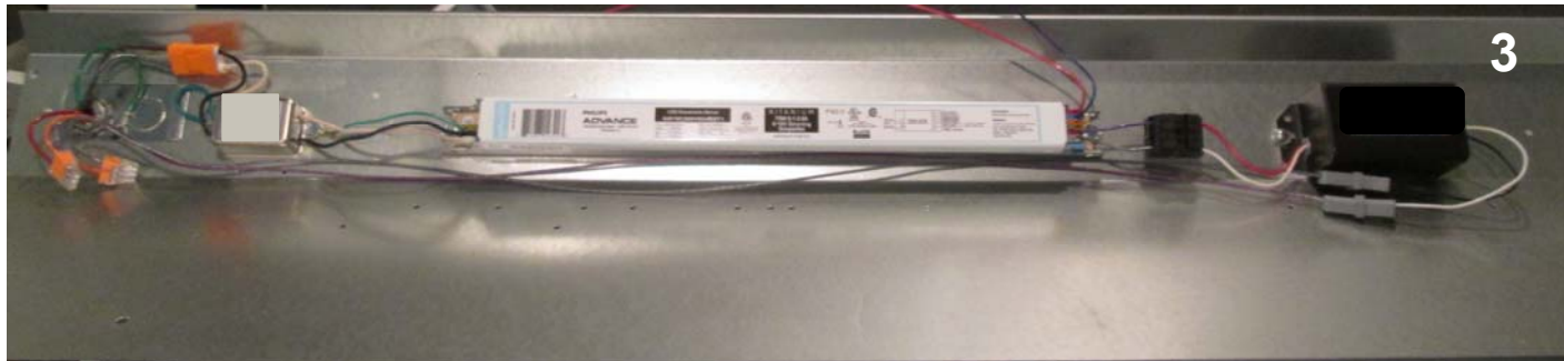
Pic 1-3: One filter is installed between main input wires and driver's input connections, and this new mounting position would make input wires shorter(Pic 1). One filter is installed between the driver's dimming connectors and control wires from conduit (Pic 2). Overall modified wiring connection and filter installation are shown in Pic 3.
