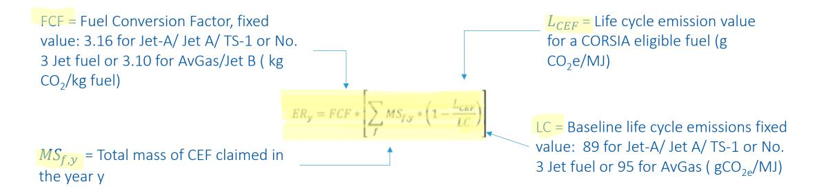
Example: If, in 2021, an operator uses 10,000 tonnes of Jet-A Fuel produced from Used Cooking Oil (Default  $L_{CEF} = 13.9g$  CO2e/MJ), the amount of emissions reductions will be:
