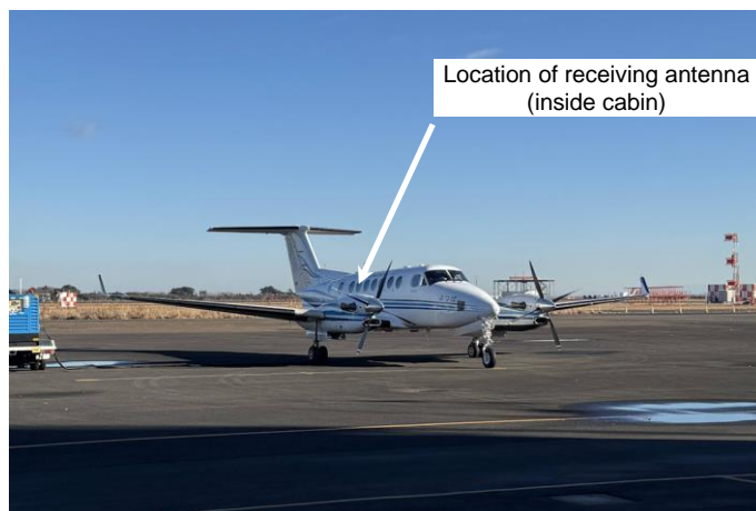
Figure 2. Beechcraft B300 aircraft (used for flight experiments) and location of the receiving antenna.
