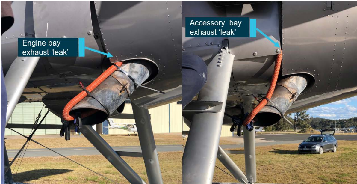
Figure 45: Simulated exhaust leak into the engine bay (left) and the accessory bay (right)
