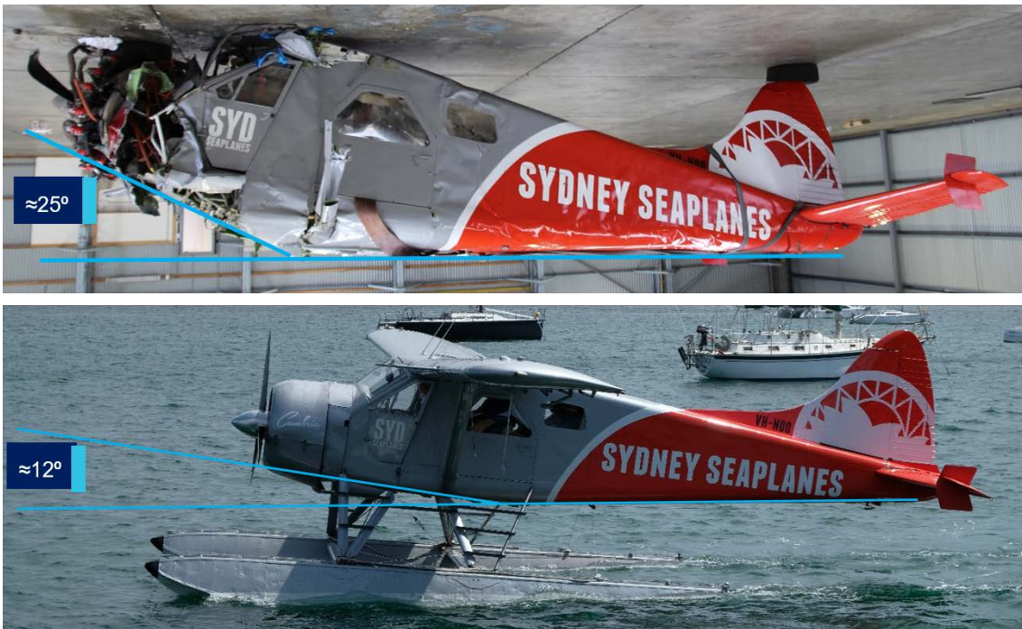
Figure 21: Engine and forward fuselage deformation post-accident (top) with pre-accident nose to rear fuselage angle (bottom)
