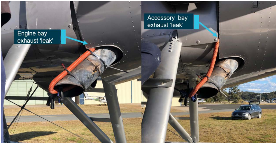
Figure 57: Simulated exhaust leak into the engine bay (left) and the accessory bay (right)
