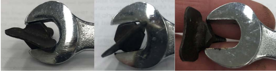
Figure 29: Spanner accessibility on AN3 modified bolt
