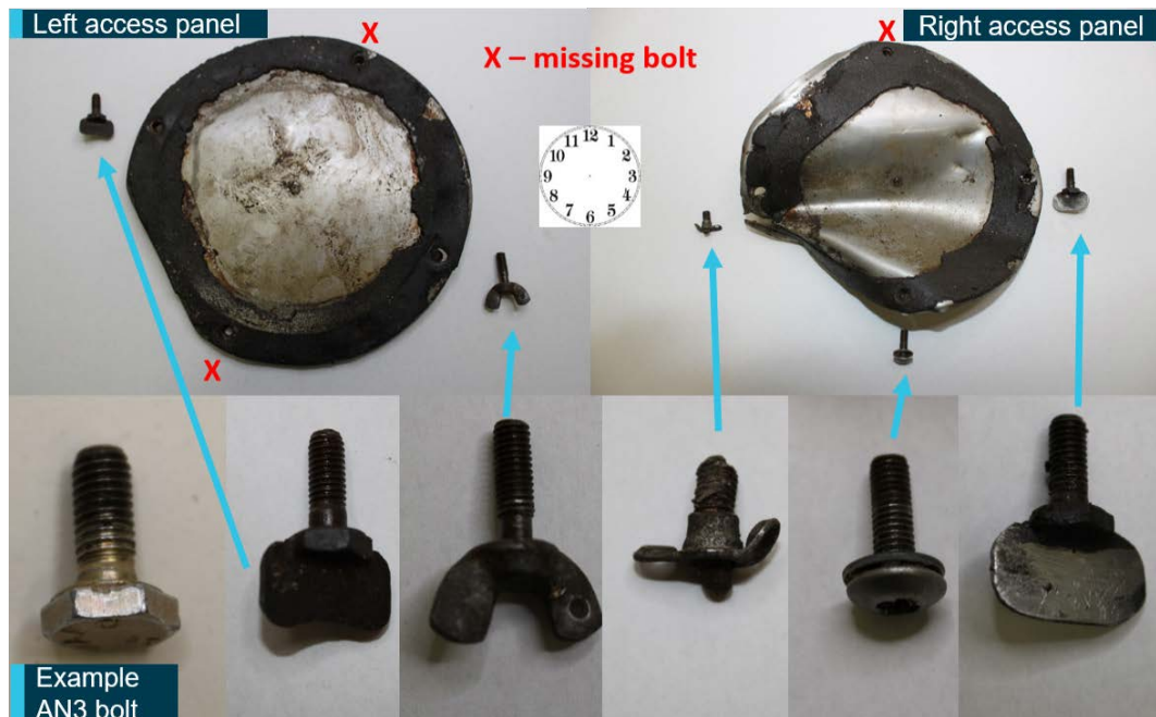
Figure 28: Magneto access panels, attaching hardware and gaskets
