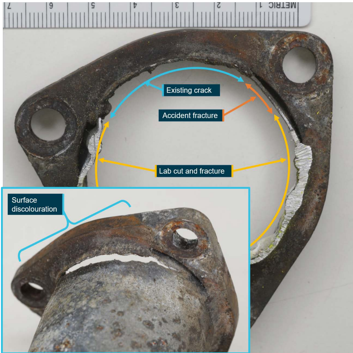
Figure 49: Cylinder number 7 exhaust flange crack (detail E)
