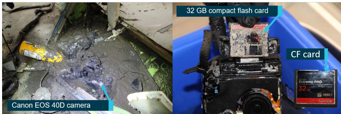
Figure 13: Passenger camera as found in the aircraft (left) and CF card removal (right)
