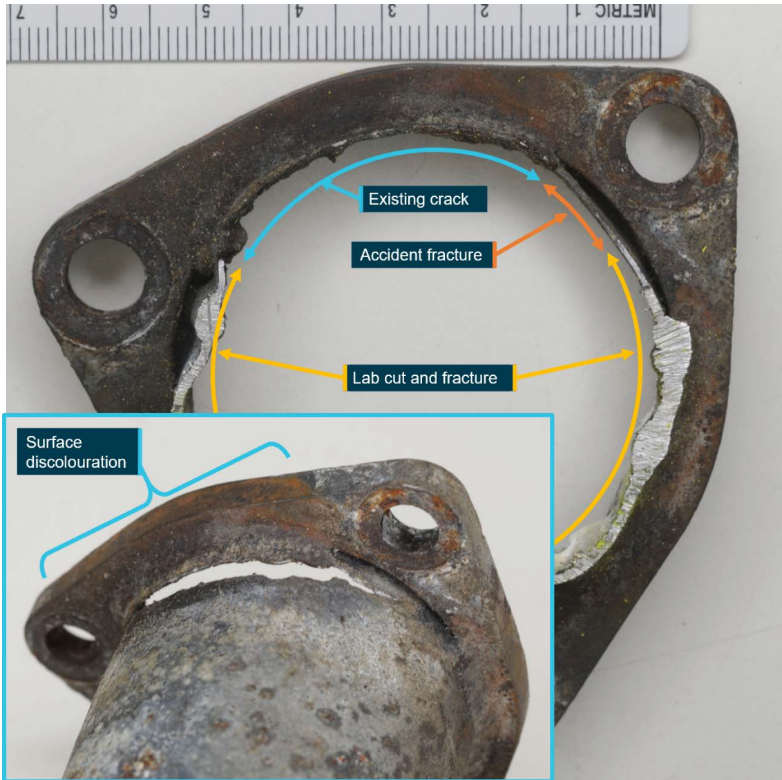
Figure 26: Cylinder 7 exhaust flange (detail E)
