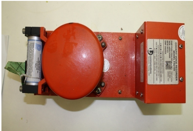
Figure 5 Cockpit Voice Recorder (CVR) FA2100 SN000274566
