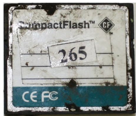
Figure 10 CompactFlash memory card (bottom view)
