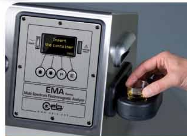
View of the EMA External Probe
