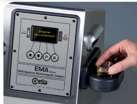
View of the EMA External Probe
