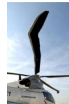
Figure 1. Prototype 3D blade profile tailoring.
