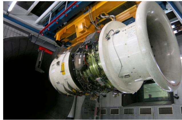
Figure 2. Single Orifice Probe nvPM Measurements in the Test Cell of SR Technics, Zurich Flughafen (Courtesy of SR Technics).
