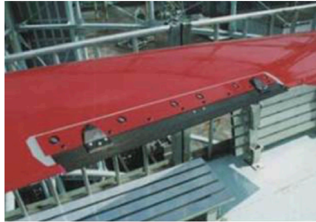
Figure 3. Full-scale rotor blade active flap test
