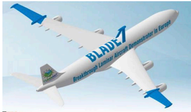
Figure 2. Integrated NLF Design Concepts Installed on A340 Wing Tips of Clean Sky 2 Flight Demonstrator 2 .
