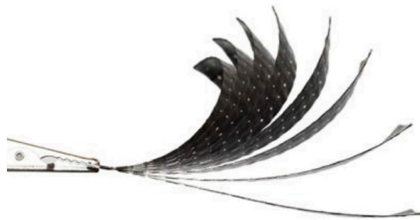
Figure 7. Programmable Adaptable Carbon Fiber (laboratory test coupon).
