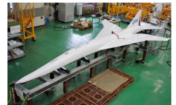
Figure 2. JAXA's Scaled Airplane – Used During Drop Test
