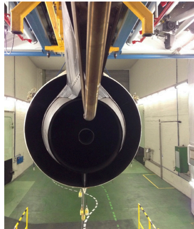
Figure 2. Turbofan Engine Seen From Behind With Tube of a Sampling Probe.
