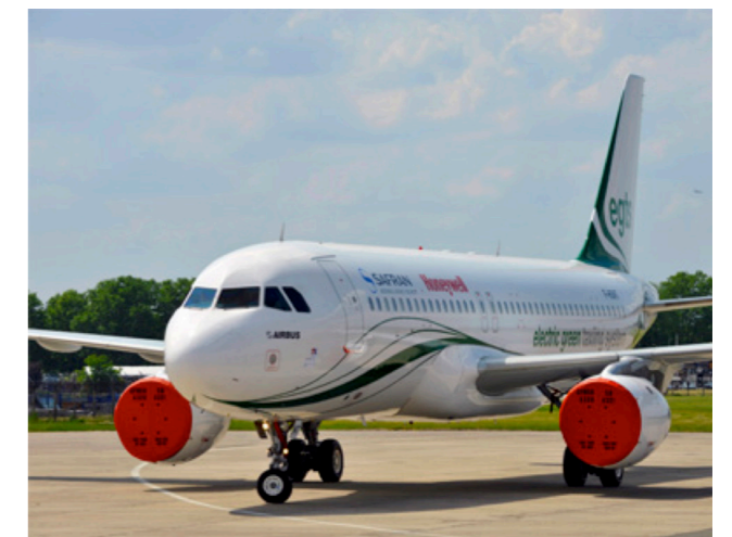
Figure 2. An aircraft with an e-taxi system installed taxiing using only the power from the APU. Source: http://articles.sae.org/12662/
