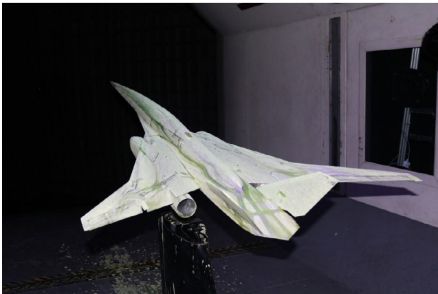
FIGURE 2: Exosonic Large-Scale Low Speed Wind Tunnel Test Surface Flow Visualization
