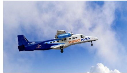
FIGURE 4: In March 2021, ZeroAvia launched the development programme for a 2MW hydrogen-electric powertrain for full-size regional aircraft
