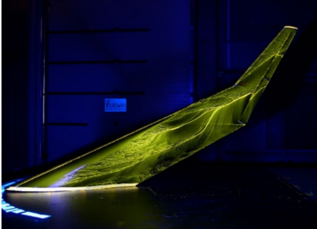
FIGURE 3: Large vortex structures appear at high angles of attack over the inner wing of the Flying V. 6
