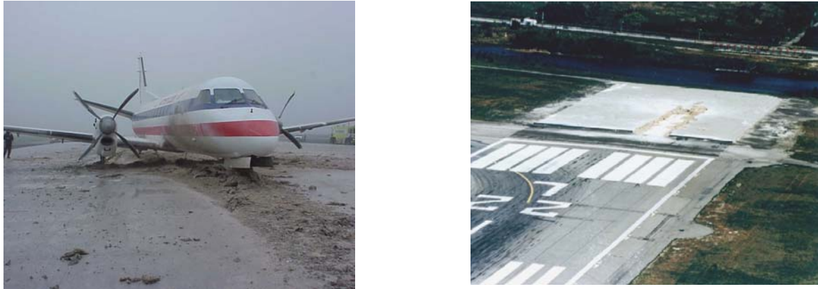
Figure 5 - Photos of EMAS off Runway 22L at JFK taken the day after the safe arrestment of a SAAB-340 overrun in June 1999 (note the surface area removed to extract the aircraft)
