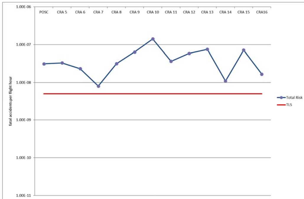
Figure 1: The total vertical collision risk estimates of the successive post-implementation CRAs on a normal scale (top figure) as well as on a logarithmic scale (bottom figure). The red horizontal lines indicate the TLS of 5.0 \times 10^{-9} fatal accidents per flight hour.
