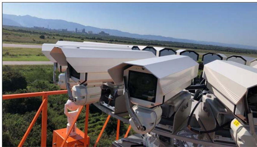
Figure 4 - R-TWR Santa Cruz camera system
