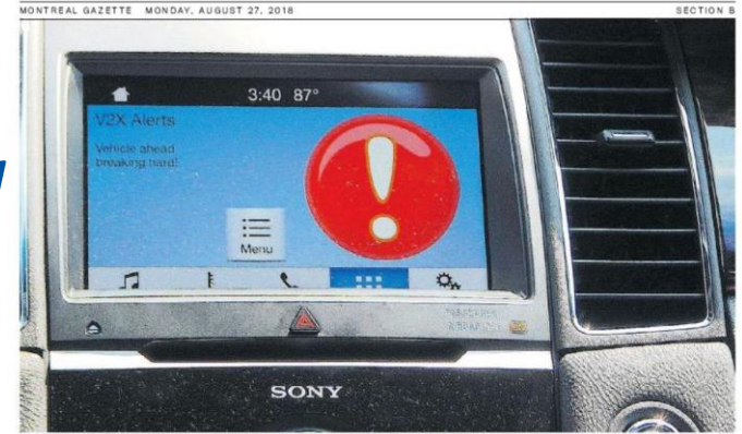
Ford's Cellular Vehicle to Everything (C-V2X) system will, among other things, warn motorists of dangerous situations ahead of them. BYRON HARRIS
