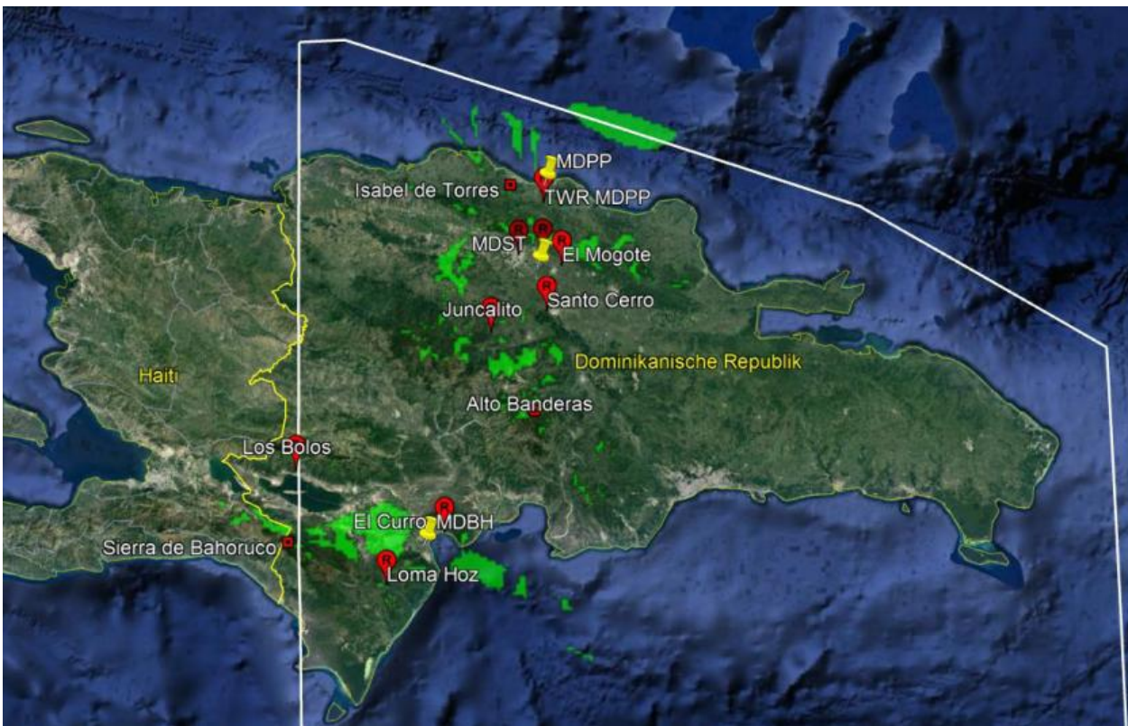
Figure 6-22: Configuration 2 - Coverage at 1000ft AGL N-situation
