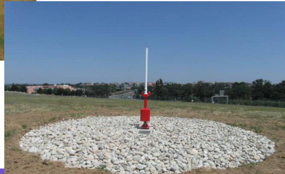
Reference Receivers antennas
