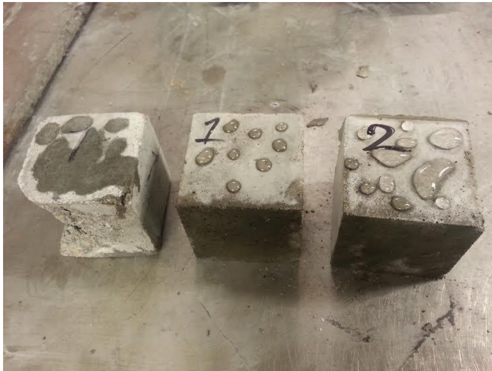
From left to right: control, 2% PTFE, and 5% PTFE modified mortar specimens
