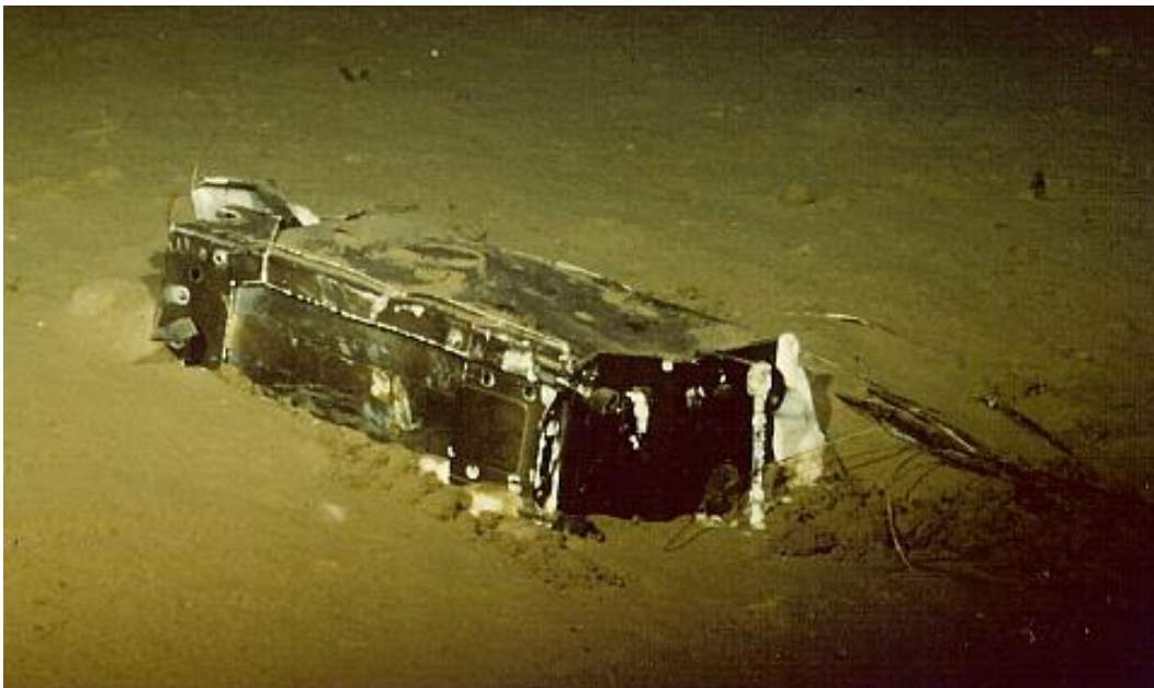
Figure I-5-7. The cockpit voice recorder of a Boeing 747 Combi photographed at a depth of approximately 4 500 m in the Indian Ocean (1987 accident)
