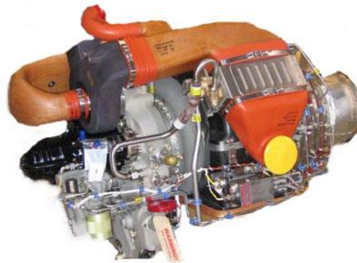
APU (Auxiliary Power Unit)
