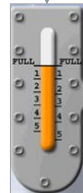
Engine oil tank sight glass reading
