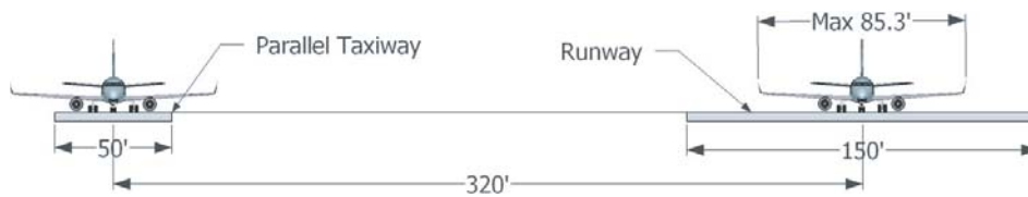
Figure A-13. Example of Runway/Taxiway Separation.
