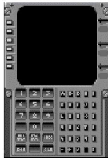
Control/Display Unit (CDU) #1
