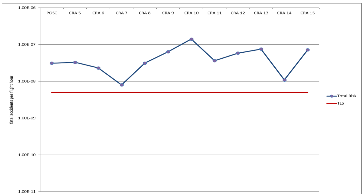
Figure 4: The total vertical collision risk estimates of the successive post-implementation CRAs on a normal scale (top figure) as well as on a logarithmic scale (bottom figure). The red horizontal lines indicate the TLS of 5.0 \times 10^{-9} fatal accidents per flight hour
