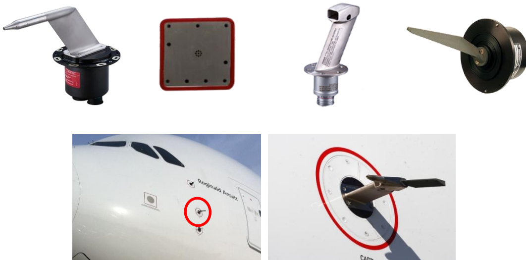
Figure 3.7 Air Data Sensors and Integrated Sensor on Airbus A380
