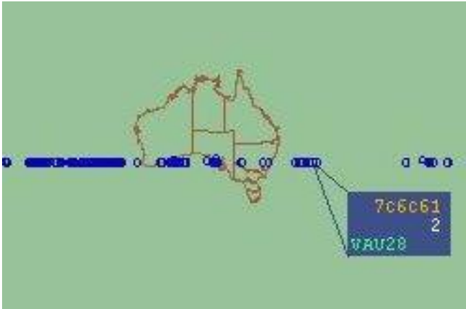
Figure 1 - Track Jumping problem with TPR901
