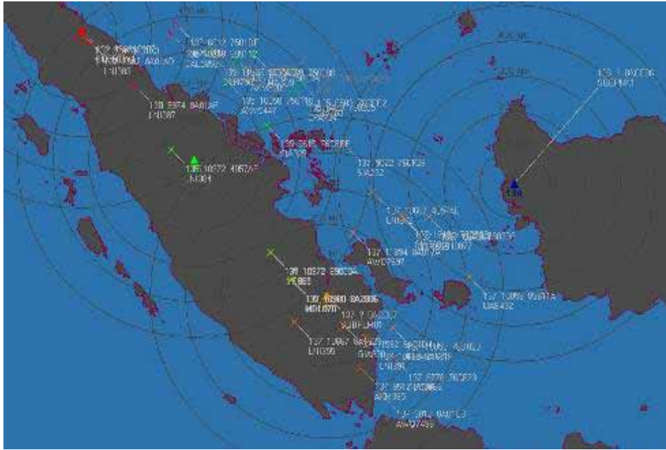
Figure 5. Aircraft detected from Era Groundstations and displayed at Era RCMS.
