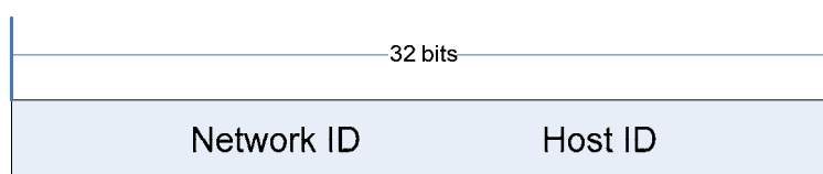
Figure 2-1. IPv4 Address Format
