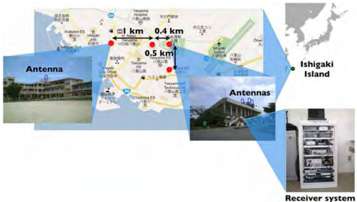
Figure A3.1. Overview of the ENRI's local area ionosphere observation system in Ishigaki Island, Japan.
